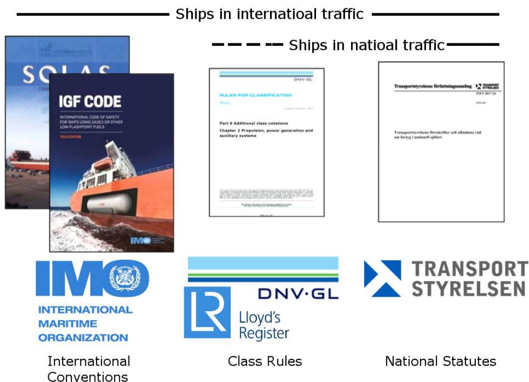
Figure 3: The layers of regulations for installations on ships and boats. The regulations from IMO are not directly applicable but influence the national statutes and class requirements. Class rules are always applicable for ships covered by the international rules and can be for ships in national traffic. Class requirements can also be used in the design and specification of ships in national traffic even though the ship may not have class certificate. The ship can, however, be built with class certificate, as was done for the new Finnish road ferry Elektra.
